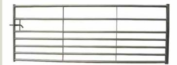
This is our most popular field gate, available in a full range of sizes, with 7 rails, D loop or spring bolt fastenings. Bracing is punched flat for added strength and reduced ear tag losses. Top and bottom rails are 44.5mm dia tube, intermediates are 30mm. Height 1143mm.
