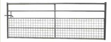
A quality field gate ideal for containing small animals and young stock. It has a sleeved box section hanging stile, 44.5mm o.d. top and bottom rails, 30mm o.d intermediates and is clad with 75 x 75mm weldmesh. Height 1143mm.
